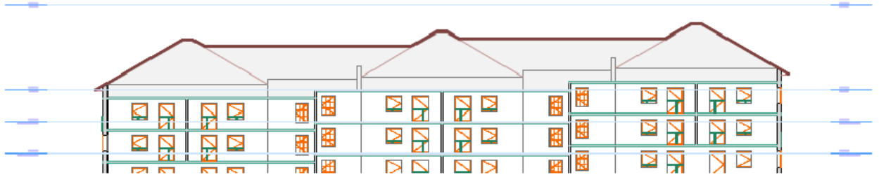
Attic space with different floor and roof levels
